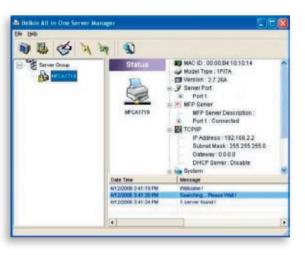
Every time you run the "Server Manager" configuration utility, click the "Search" icon on the tool bar. The configuration utility will delay for several seconds because the utility is using the system's available network protocols to search for all Print Servers on the network. All available Print Servers will be listed under "Server Group" on the left side of the window.
